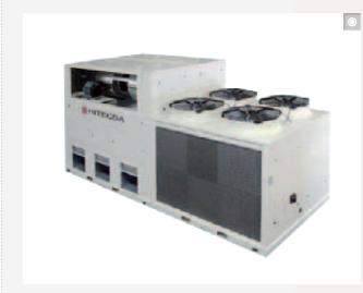
The RXCA/RXCBA RCF series units are self-contained compact rooftop units that are specially designed for installation on rooftops, roof terraces or in any other outdoor location with air distributed treated in ducts. The heat recovery system uses an additional cooling circuit as a heat exchanger. This purpose of this new circuit is to transfer the energy from the exhaust air to the new ventilation air.
