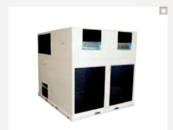
The RCCA/RCCBA RCF series units are self-contained compact roof top units with centrifugal fans on the two sections, suitable for indoor installation. Air distribution is channelled through ducts. The heat recovery system uses an additional cooling circuit as a heat exchanger. This purpose of this new circuit is to transfer the energy from the exhaust air to the new ventilation air.
